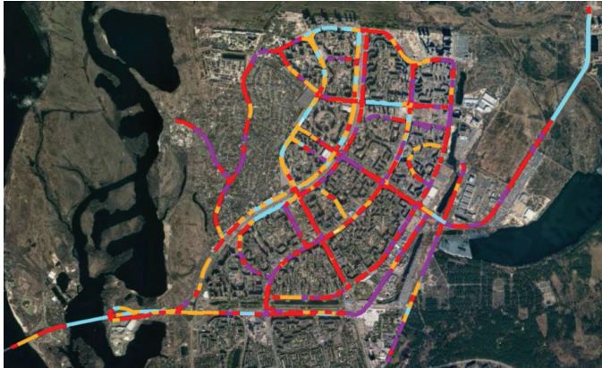
Figure 3 Cartogram of IRI values, Troyeshchyna, Desnyansky district, Kyiv, as of September 2024, built by the RoadLab Pro software complex and processed in Google Earth
