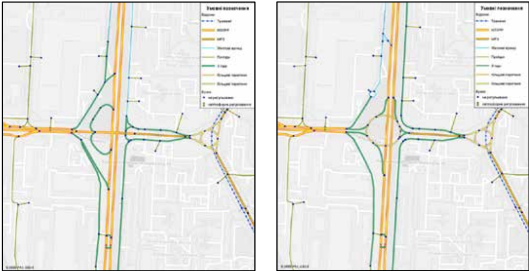
Fig. 7. Project solutions for the intersection to establish an interchange: semi-“clover leaf” (left) and the roundabout with flyover (right)
